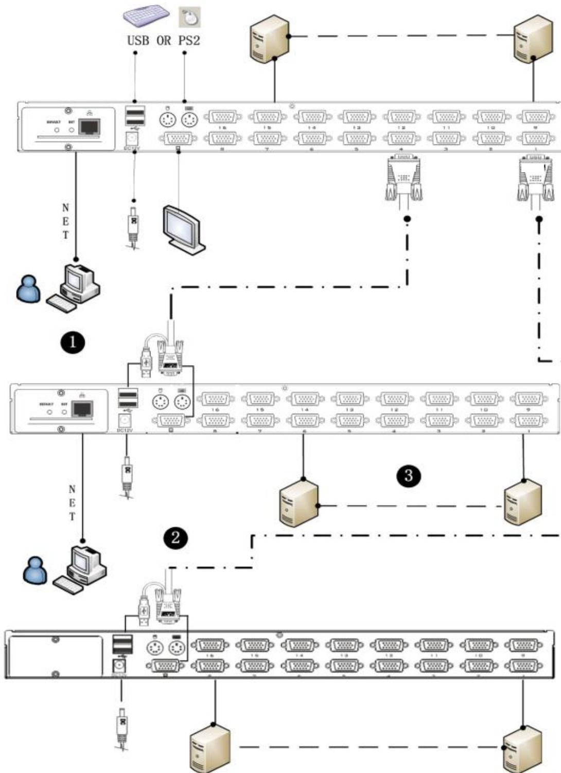
The cascade mode, it's the same method of keyboard, mouse and computer connections as stand-alone connection, this part will not repeat them, the number part of the description is as follows:
