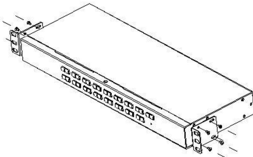
3. Install the KVM switch with the mounting plate attached to the rack, and align the mounting hole of the mounting plate with the mounting hole on the rack. Use the rack mounting screws in the mounting bracket to secure the mounting plate to the front end of the rack tight.
