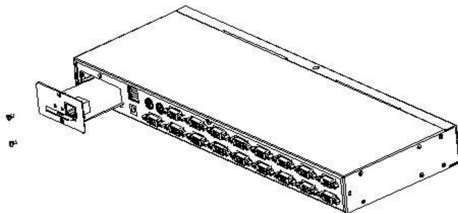
4. After finishing the installation of the IP module, please follow the instructions of the IP module user manual to install the software and network IP configuration of the device before connecting the network cable to the switching equipment. Then, you can access the network to log in to use. (For details, refer to the IP module's user manual.)
