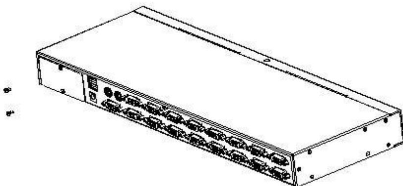
1. After removing the blank, you can see the cavity which install the IP module, keep the screws which are removed down.
