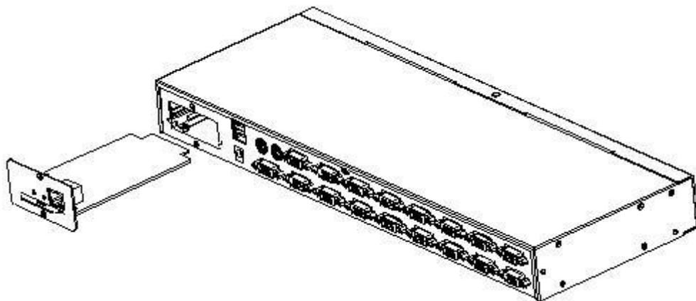
3. Push the IP module to the bottom, and then tighten the IP module with the two screws which removed from the front panel.
