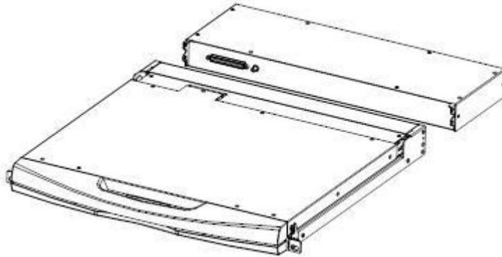
4. Replace the KVM module at the rear of the LCD. Fix the screws in the corresponding screw holes as shown in the figure, and then fix the whole machine in the cabinet according to the corresponding steps.
